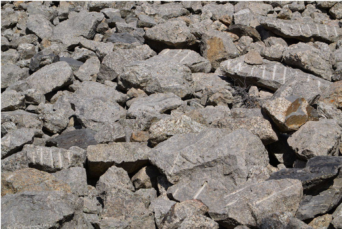
Rubble from sculpting activity on Mt. Rushmore. Note the drill and chisel marks.
